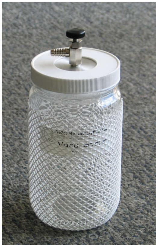
The Vacu-Storr series of glass vacuum containers were developed to store materials which are sensitive to moisture, oxygen, and other gases found in the environment. It can also be used to protect the environment from the contents. Also available in stainless steel. The Vacu-Storr is capable of nearly reaching the vacuum level of  $10^{-4}$  torr. With a higher conductance valve and capable pump  $10^{-6}$  torr is achievable.
