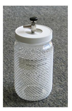
The Vacu-Storr series of glass vacuum containers were developed materials which store sensitive to moisture, oxygen, and other gases found in the environment. It can also be used to protect the environment from the contents. Also available in stainess steel. The Vacu-Storr is capable of nearly reaching the vacuum level of  $10^{-4}$ torr. With a higher conductance valve and capable pump 10<sup>-6</sup> torr is achievable.
